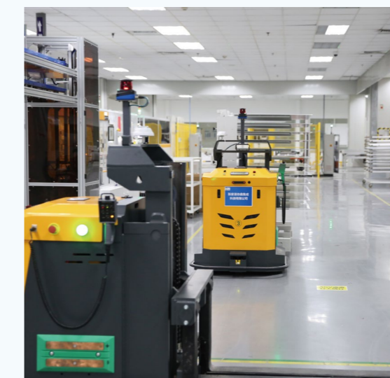
AGV automatic scheduling of feeding
